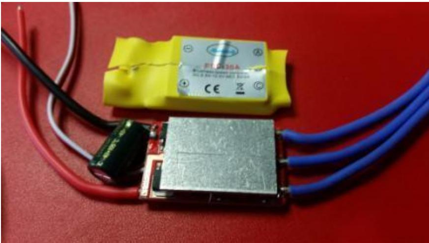
Standard ESC's have a metal plate attached to the semiconductors which is then wrapped in heat-shrink. This is a satisfactory heat sinking arrangement if the ESC is overrated for the motor and if the motor is not run for long periods at high power, and if there is adequate cooling air passing by. That is a lot of ifs....
