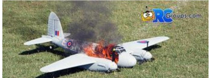
Such a fire is directly related to the battery because that is the source of the heat which is essential for any fire to develop. There have been a couple of ESC fires (that I know about) so I thought we could look at the causes and preventative measures that can be taken. ESC heating can be a common cause of so-called radio failures, the reasons for which will become apparent when we look at how these things work.
