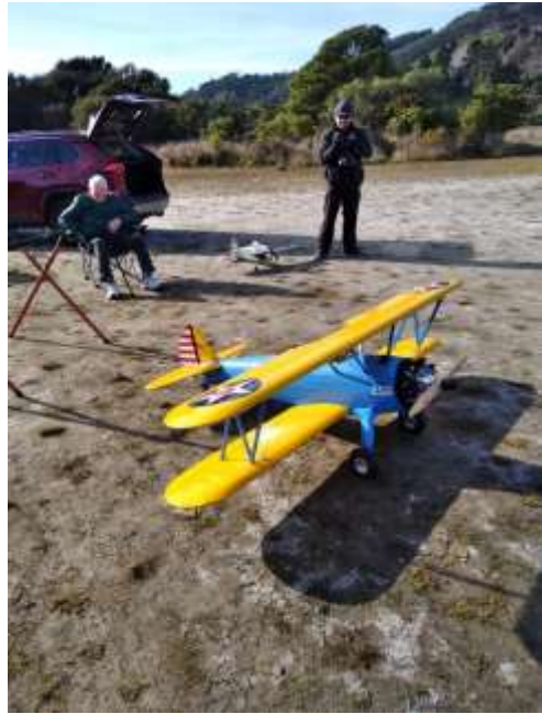
Wayne's latest maiden. 100cc UMS 5-Cylinder Radial powering his Boeing Stearman. We're all waiting to hear this out at the field soon.
